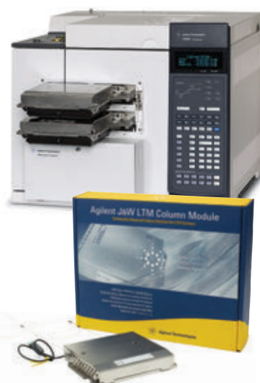
LTM II standard format with 5 in column toroid
